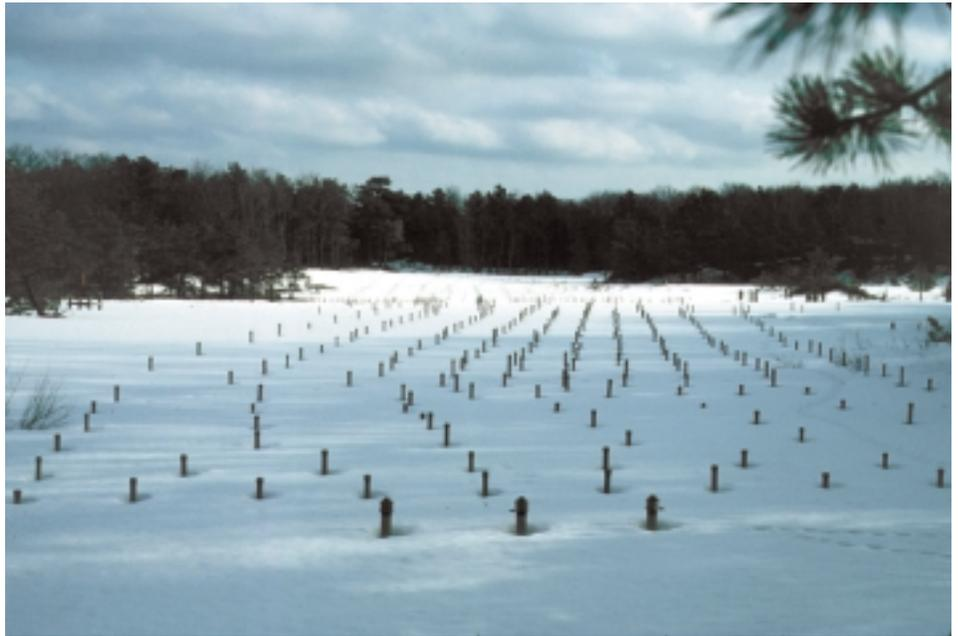
An array of vertical multi-point sampling devices installed to monitor small-scale subsurface geochemical heterogeneities in a contaminant plume at the Cape Cod, Massachusetts, research site. Knowledge and models developed at this site are employed at many sites with sparse data.
